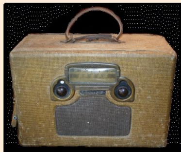
1942 portable Farnsworth radio that could be operated off an internal battery pack or by plugging it into AC
